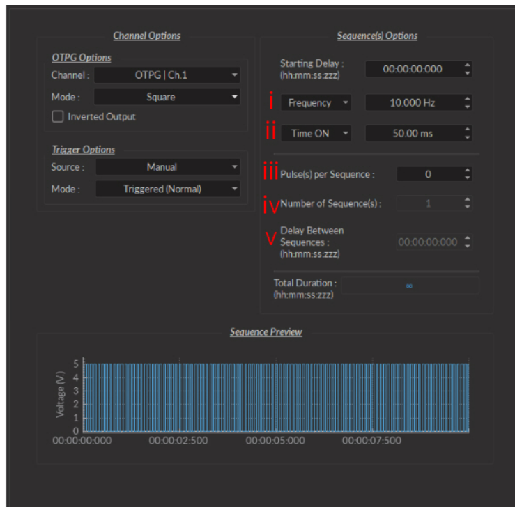
Figure 3.65: Channels Configuration, Square Interface
