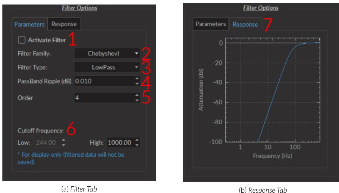
Figure 3.23: Linear Mode Filter Options
