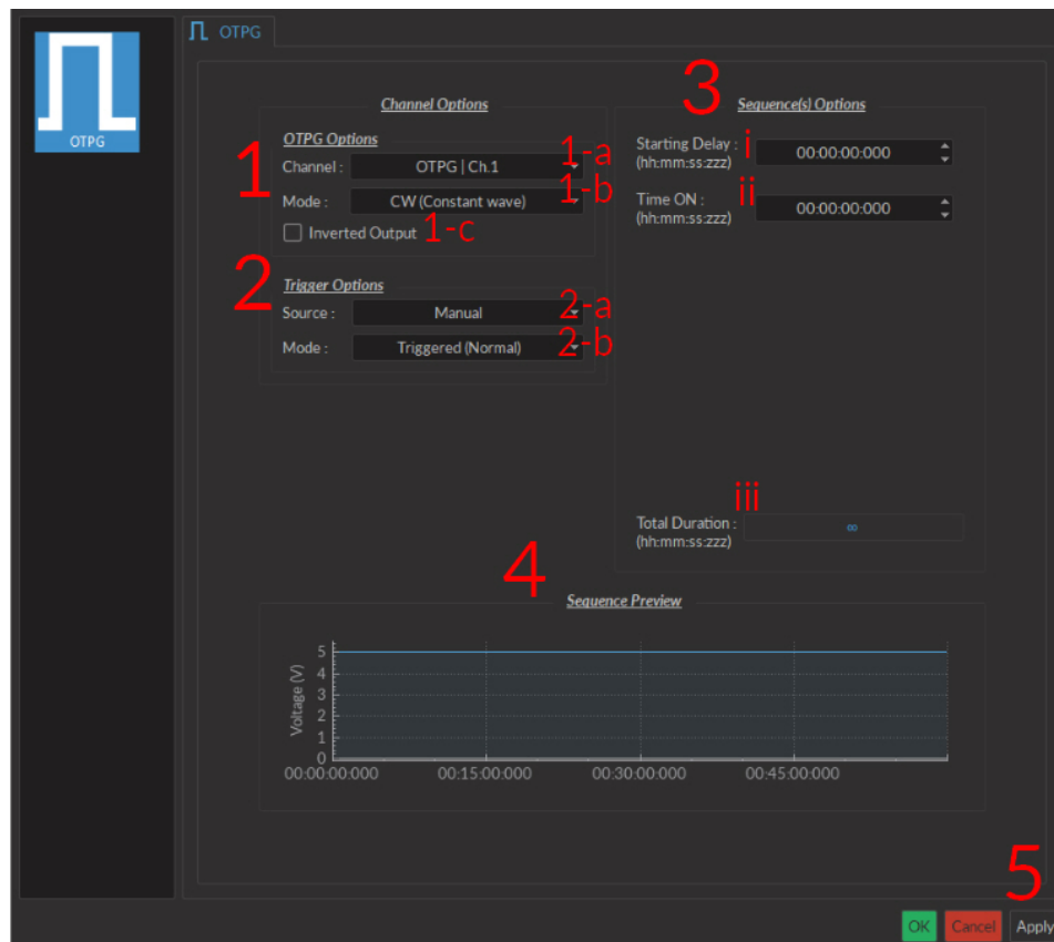
Figure 3.64: Channels Configuration, Continuous Wave Interface
