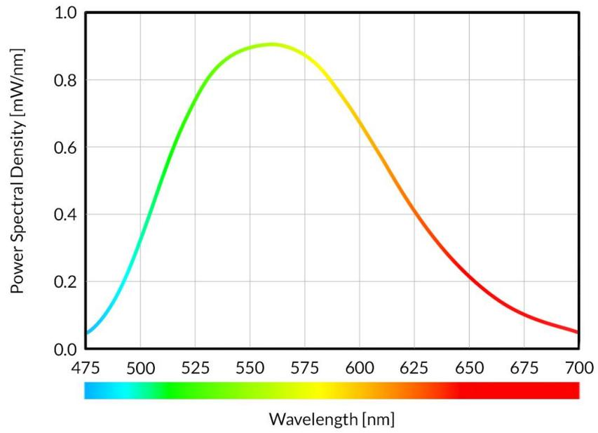
Figure 2.1: Output Power Spectral Density of a  $\star$ LISER<sup>TM</sup> Fiber Light Source using 200  $\mu\text{m}$ , 0.53 NA Fiber
