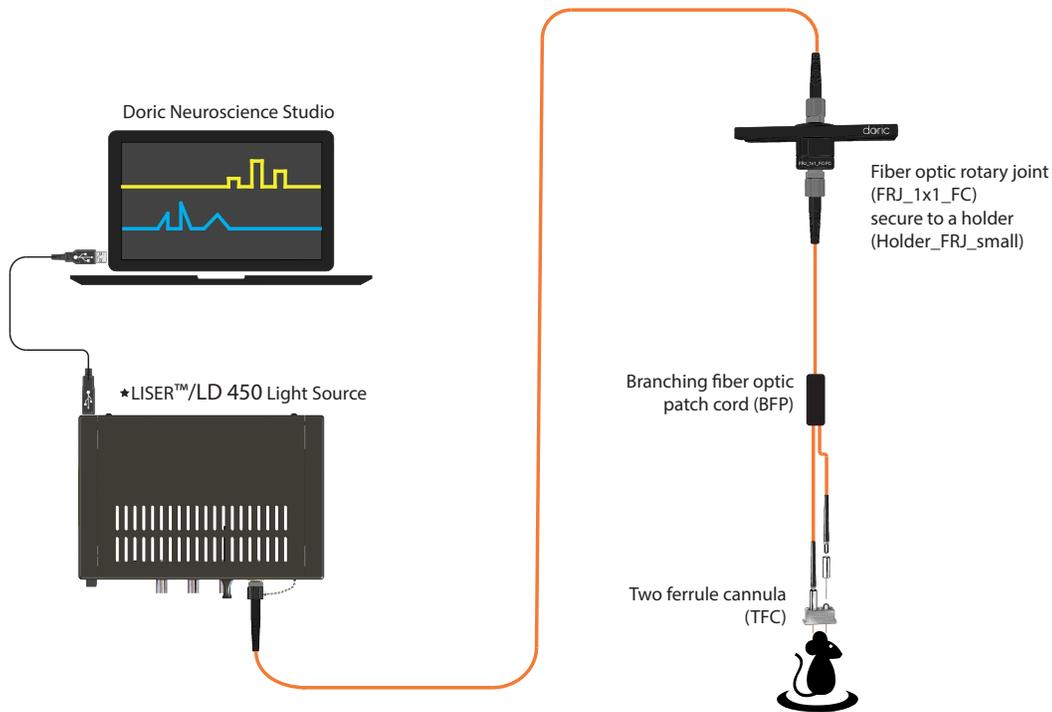
Figure 3.1: System using a ★LISER™ & LED/LD Light Source
