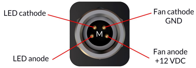
Figure 4.1: M8 Connector Pinout
